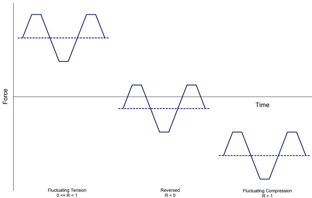
Figure 3 – Varying force ratio according to BS EN 2987:2009.
