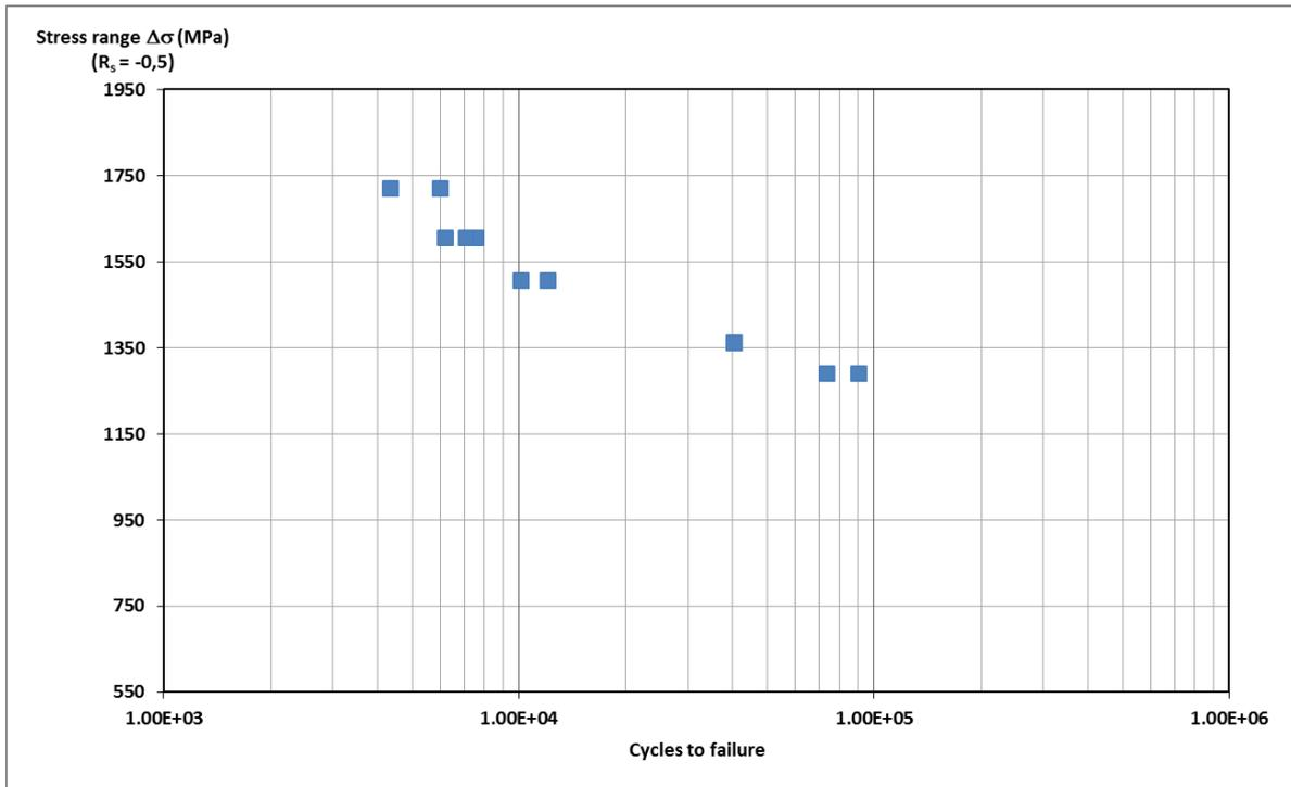
**Figure 5: Typical S-N diagram according to BS EN 2987:2009.**
