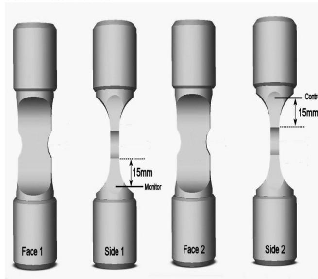
**Figure 9: Schematic stage 3 TC arrangement (2 TC's).**
