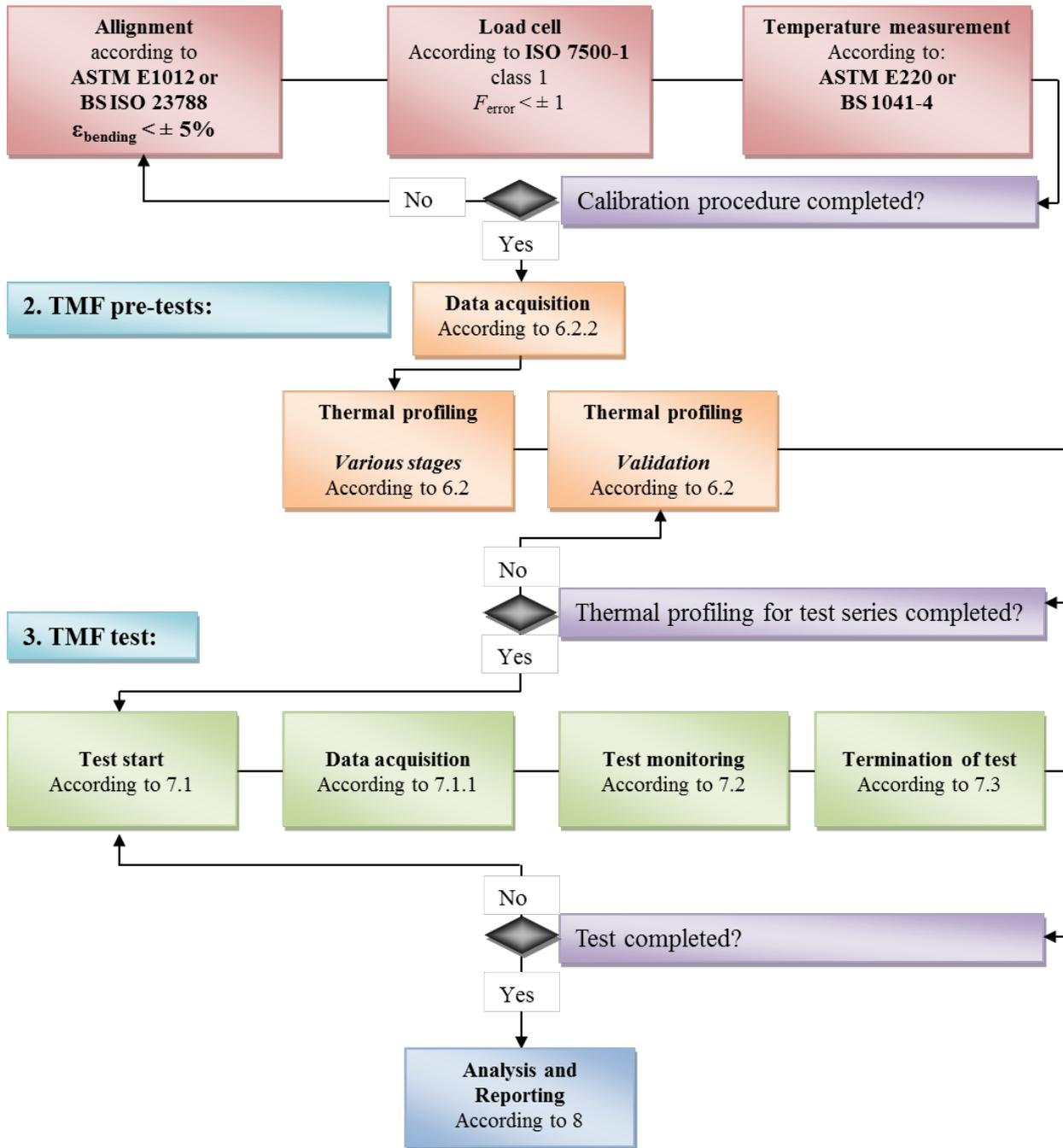
Figure 1: A flow diagram outlining the various steps in undertaking a force-controlled TMF test according to this code of practice<sup>1</sup>.
