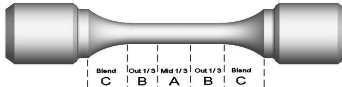
**Figure 6: Failure locations along the gauge length of cylindrical or square section plain specimens.**
