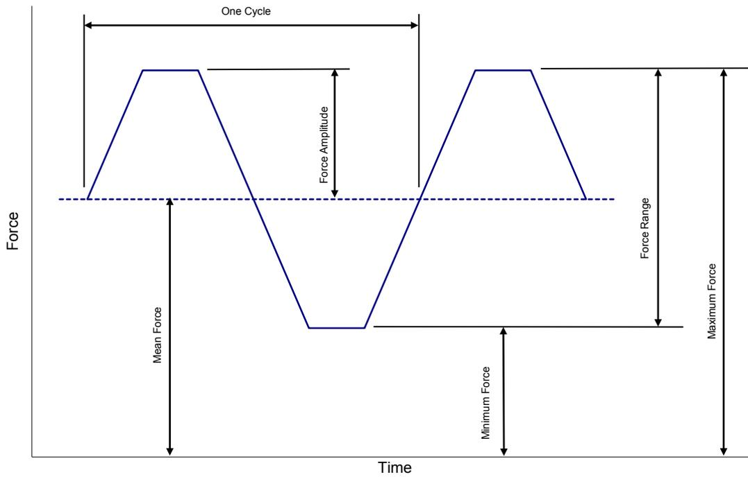
Figure 2 – Fatigue force cycle according to BS EN 2987:2009.
