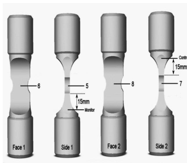
**Figure 8: Schematic stage 2 TC arrangement (6 TC's).**
