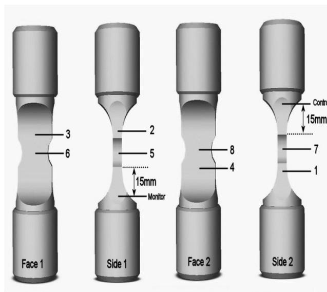
**Figure 7: Schematic stage 1 TC arrangement (8 TC's).**
